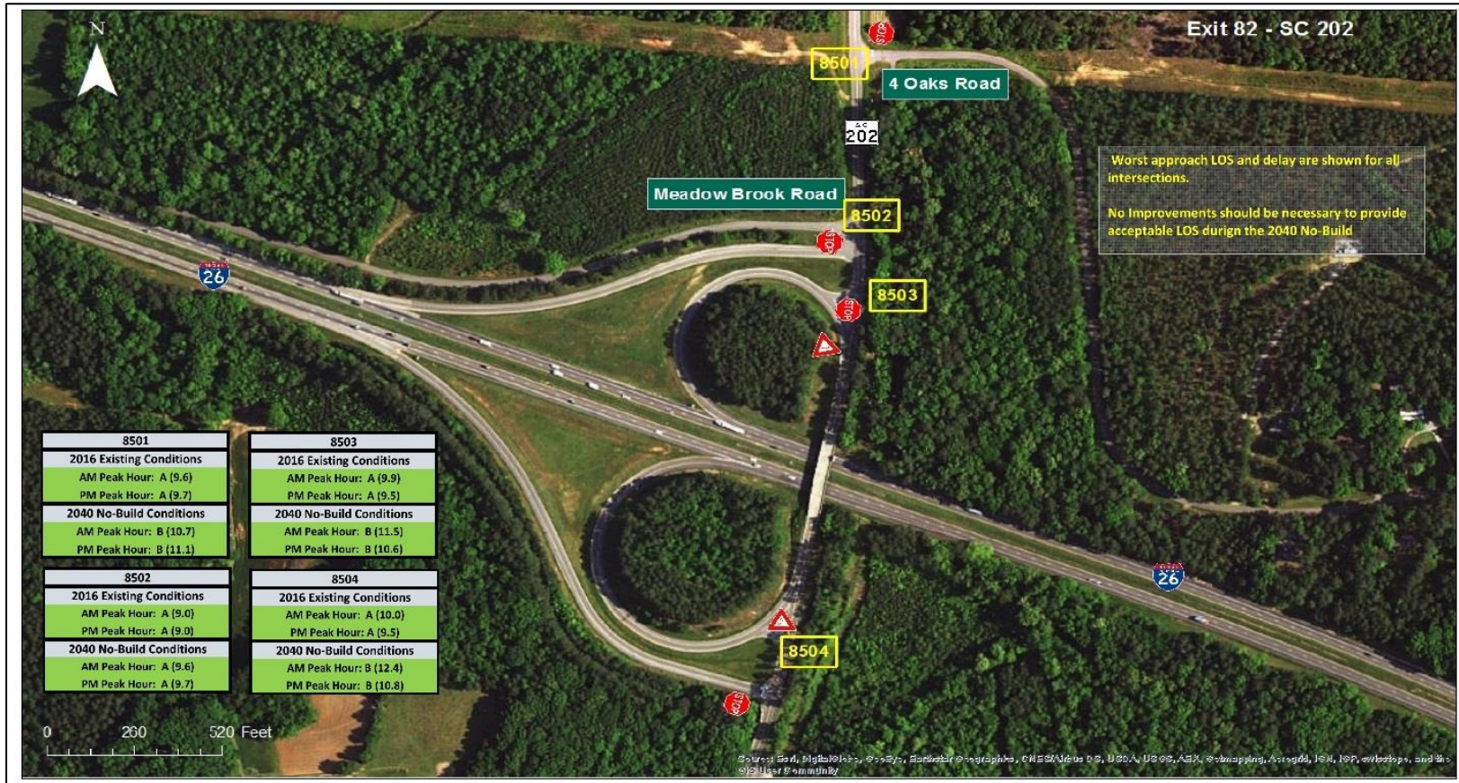
Source: Figure 74, Interstate 26 Widening Traffic Analysis Report Figure 14. Exit 85 – SC 202 Interchange Intersection LOS Summary
